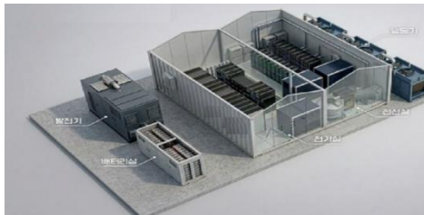
Figure 6-1. Modular AI Data Center Rendering
